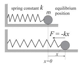
**Figure 7:** A mass on a horizontal spring. Top: The mass in it's equilibrium position with the spring unstretched. Bottom: The mass is displaced from equilibrium by an amount x, leading the spring to exert a force -kx pulling it back towards the equilibrium point.
