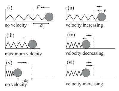
**Figure 8:** Snapshots of a mass oscillating on a spring. The mass is drawn back to  $x = a_0$  then released, leading to oscillations. Double headed arrow indicates force, single headed arrow indicates velocity. Further description in the main text.
