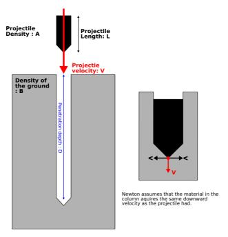
**Figure 6:** Diagram of a bullet pushing into the ground. Left: The bullet carves out a prismatically shaped column. Right: Newton assumed that all the material moved out of the way of the bullet gained a downwards velocity v equal to the initial velocity of the bullet.
