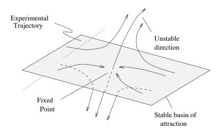
Figure 4.2: Schematic representation of RG flows in a high-dimensional space. Fixedpoints describing ordered or disordered phases generally have basins of attraction with dimensions equal to that of the space of potentials. Fixed points describing critical points have a basin of attraction of lower dimensionality.
