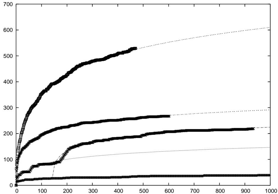
*Teaching point number as a function of teaching iterations for bulk density Silicon at 2000K, 3000K, 4000K and 5000K with a 0.25eV teaching threshold.*
