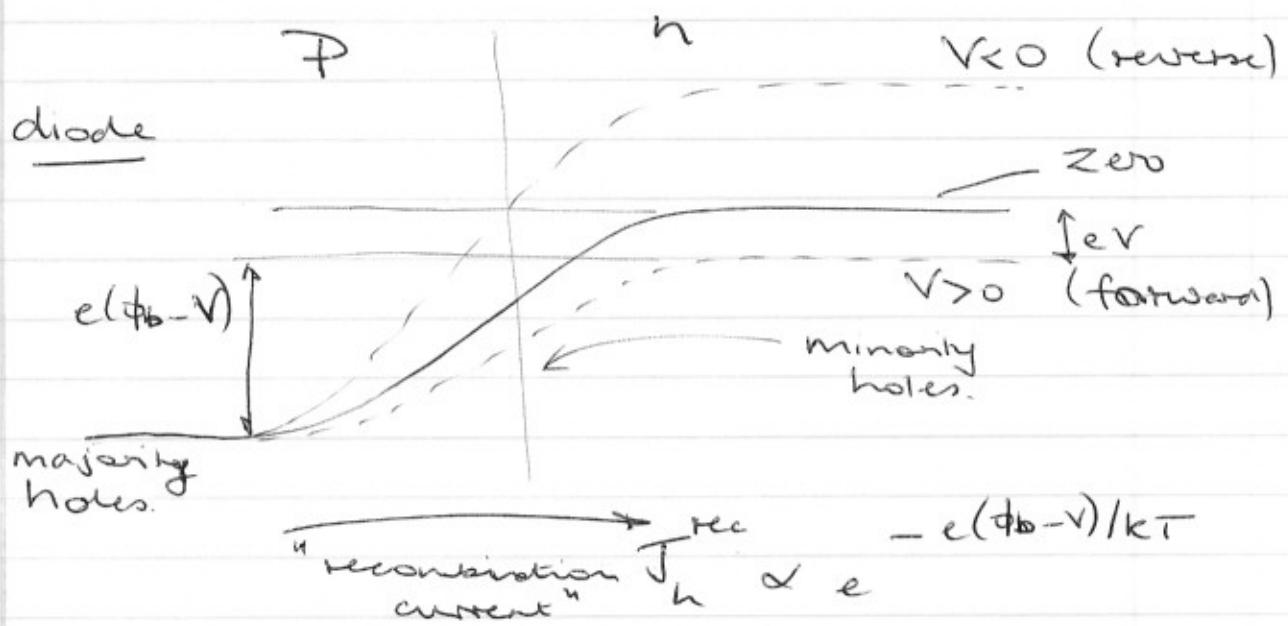
Balanced by hole "generation current" from minority holes
