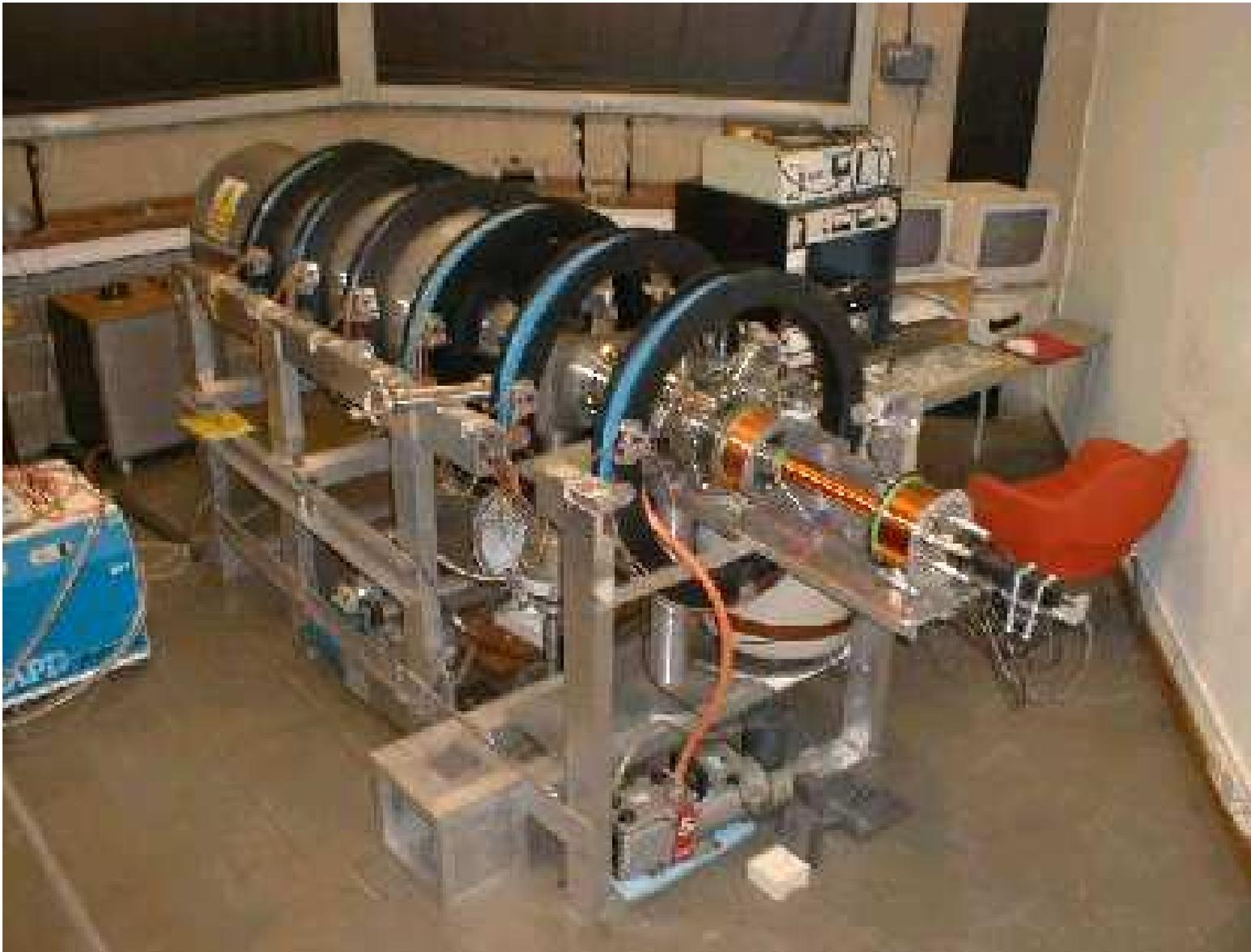
*Magnetically confined positron beam for DOBS experiments at the University of Bath*
