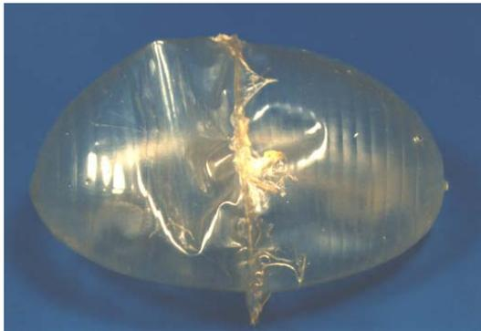
**Figure 3.7. (a)** A polyurethane ventricle made by gluing two half ventricle forms together with a solution of DMAC and polyurethane. **(b)** The male resin former and the female mould it was cast from.
