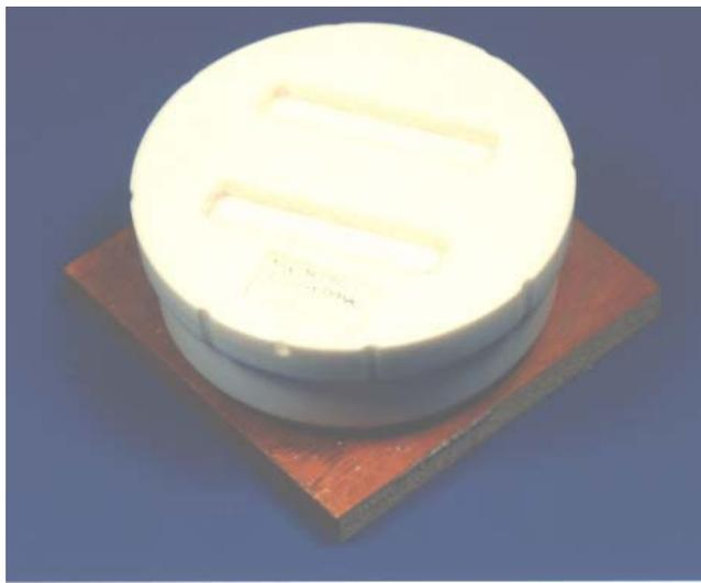
**Figure 3.6.** Teflon dipping bowl with a screw top lid for storing polyurethane dissolved in DMAC. The large width of the bowl allows artificial ventricle sized geometries to be dipped in the solution.
