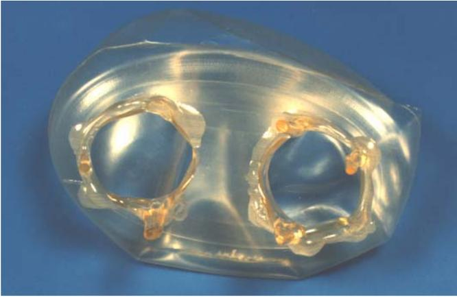
Figure 3.9. (a) The base of a polyurethane ventricle produced by coating the inside walls of a female mould with polyurethane solution. (b) A view of the ventricle showing the tear along the seam.
