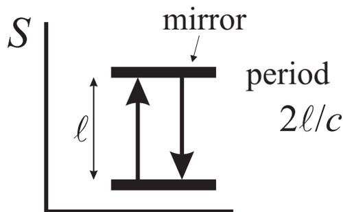
**Figure 5:** Measuring time using a light clock — a beam of light bouncing between two mirrors.
