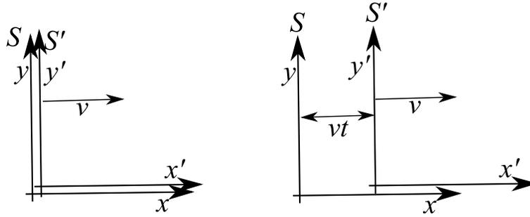
**Figure 3:** Left: Two frames  $S$  and  $S'$  in the standard configuration at  $t = t' = 0$ , at which point the two frames lie exactly on each other, although  $S'$  is moving at a speed  $v$  with respect to  $S$ . Right: A time  $t$  later  $S'$  has moved a distance  $vt$  in the  $x$  direction.
