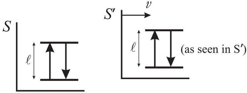
**Figure 6:** Two light clocks, one (left) stationary in  $S$  and one (right) stationary in  $S'$ , both drawn as seen in the frame they are stationary in.
