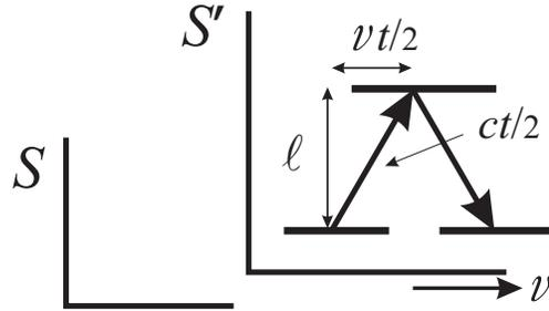
**Figure 7:** The light clock that is stationary in  $S'$  as seen according to an observer in  $S$ . The clock moves with a speed  $v$  and therefore travels a distance  $vt$  in one period of the clock.
