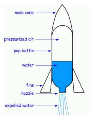
Figure 23: A rocket consisting of a soda bottle filled with water and compressed air.
