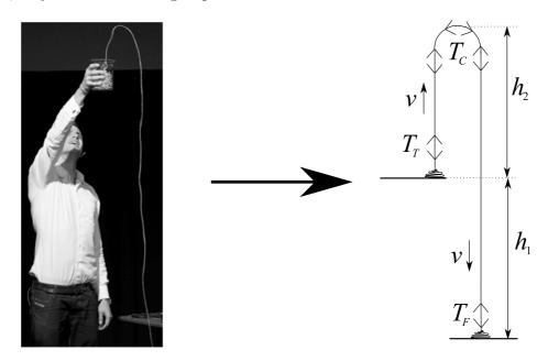
Figure 11: Photo and diagram of a chain fountain
