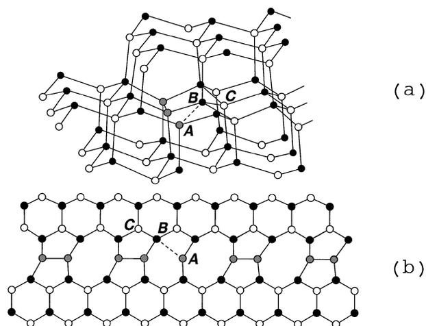
FIG. 1. (a) Three-dimensional view of a 30° partial dislocation, with a soliton domain wall, and (b) schematic drawing of the same in the (111) plane. The grey circles represent the atoms in the central core of the dislocation.
