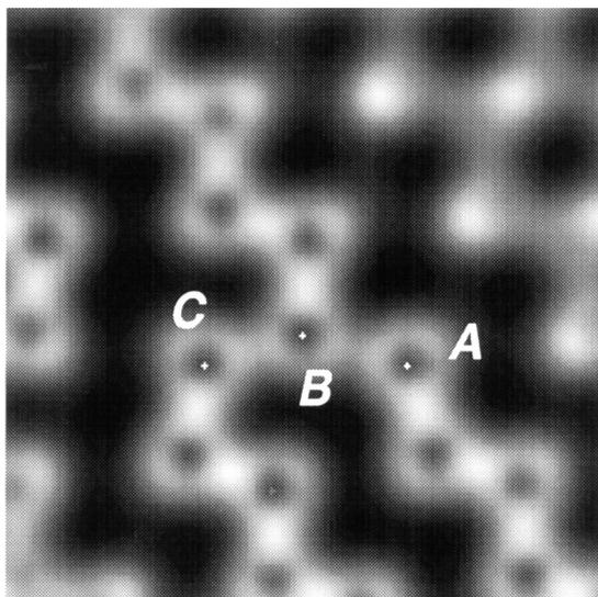
FIG. 4. Two-dimensional slice of the total charge density from our *ab initio* calculation, through the plane containing the atoms *A*, *B*, *C*, as labeled in the previous figures. The new *A-B* bond is nearly as pronounced as the bulk *B-C* bond, which is clearly weakened compared to the other (vertical) bulk bond of atom *B* seen in the figure.
