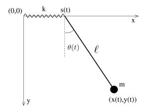
Let us call s(t) the instantaneous horizontal displacement of the hinge from the origin (i.e., the fixed point of the spring).
