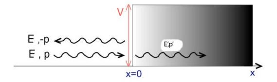
• Consider plane wave, unit amplitude, energy E, momentum  $p \, \hat{e}_3$ , and spin  $\uparrow (\chi = (1,0))$  incident on potential barrier  $V(\mathbf{x}) = V \theta(x_3)$
