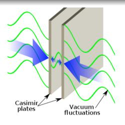
Consider two metallic plates, area A, separated by distance d – quantization of EM field leads to vacuum energy/unit area
