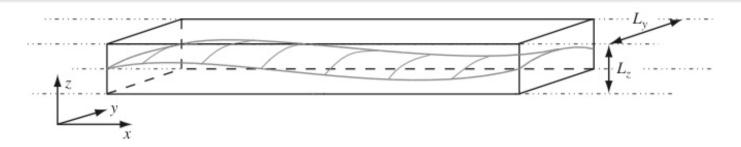
• For waveguide, general vector potential configuration may be expanded in eigenmodes of classical wave equation,
