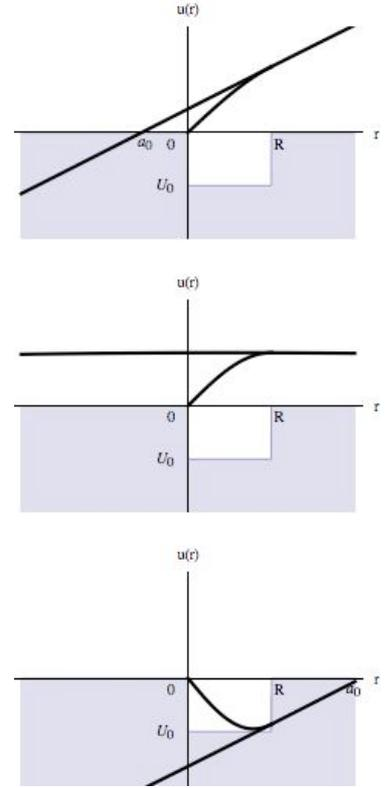
Scattering wavefunction,  $u(r)$ , for three-dimensional square well potential for  $kR = 0.1$  and  $\gamma = 1$  (top),  $\pi/2$  (middle) and  $2$  (bottom). Note that the scattering length,  $a_0$  changes from negative to positive as system passes through bound state.
