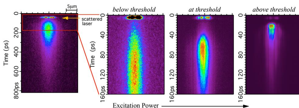
*Figure:* Temporally resolved interferograms for increasing excitation powers away from the autocorrelation point. The appearance of interference fringes at the threshold shows the transition from an incoherent to a coherent state of the polaritons. The “acceleration” of the dynamics is evidenced by the temporal shrinking of the response of the system.
