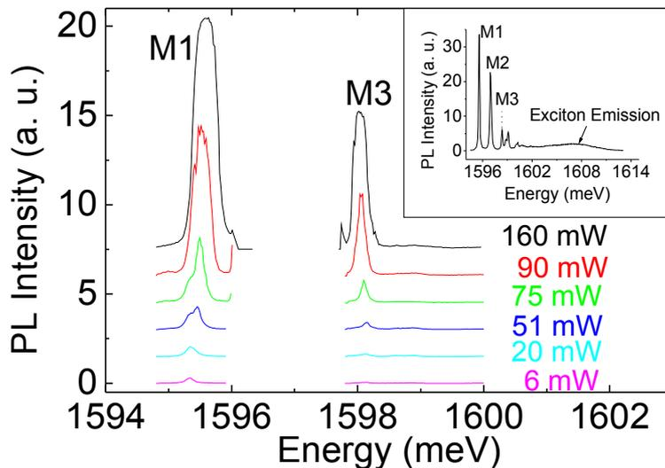
Fig 1: Emission spectrum from a 3.6  $\mu\text{m}$  square pillar under excitation resonant to M2 at 10 K. Inset: Typical photoluminescence spectra from such a square pillar under non resonant excitation.
