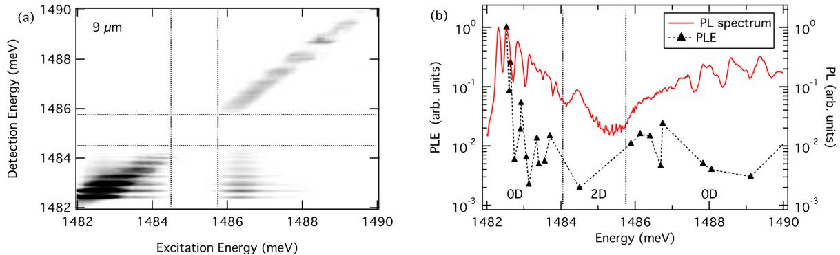
FIG. 1: PLE experiments on a 9  $\mu\text{m}$  diameter mesa. (a) : image plot, (b) : spectrum and comparison with photoluminescence spectrum. The dotted lines separate planar from confined polariton energy ranges. The relaxation down to the lowest energy states and their relative intensities suggest an efficient thermalization process.
