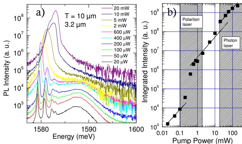
Fig: a) Emission spectra measured under non resonant excitation on a  $3.2 \mu\text{m}$  micropillar; b) Integrated intensity measured on the lower energy mode as a function of the excitation power. Shaded areas indicate the excitation range for polariton lasing and for photon lasing.
