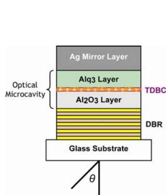
Figure 1: Device design of polaritonic structure. Microcavity consists of a DBR and a silver mirror layer. On top of the J-aggregate layer, a film of the small molecule Alq<sub>3</sub> is thermally evaporated.
